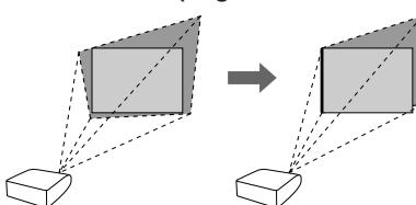
Correzione della deformazione trapezoidale orizzontale (Regolazione con
